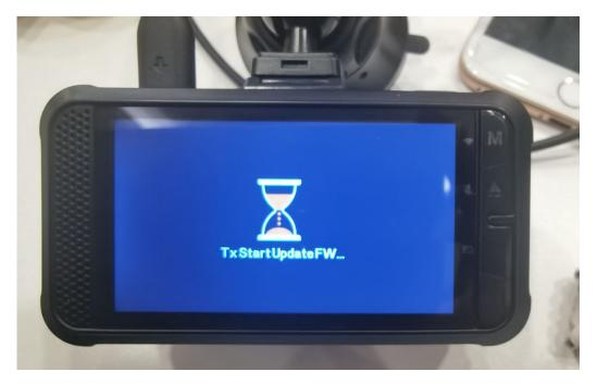
4. After the software is updated successfully, it will return to the recording interface and start recording automatically.
